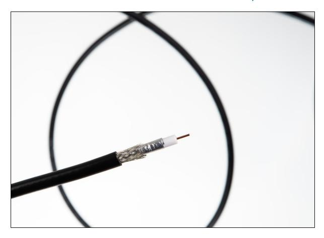
The Van Damme Enhanced Performance HD Vision coaxial is based around the industry standard RG6/U. Its precision construction ensures that electrical performance is optimised, ensuring trouble free performance with SMPTE 424M and 292M HD-SDI signals as well as SDI and analogue video. Also suitable for SMPTE 425M 6G and dual link 12G UHD use and short 12G patchcords.
